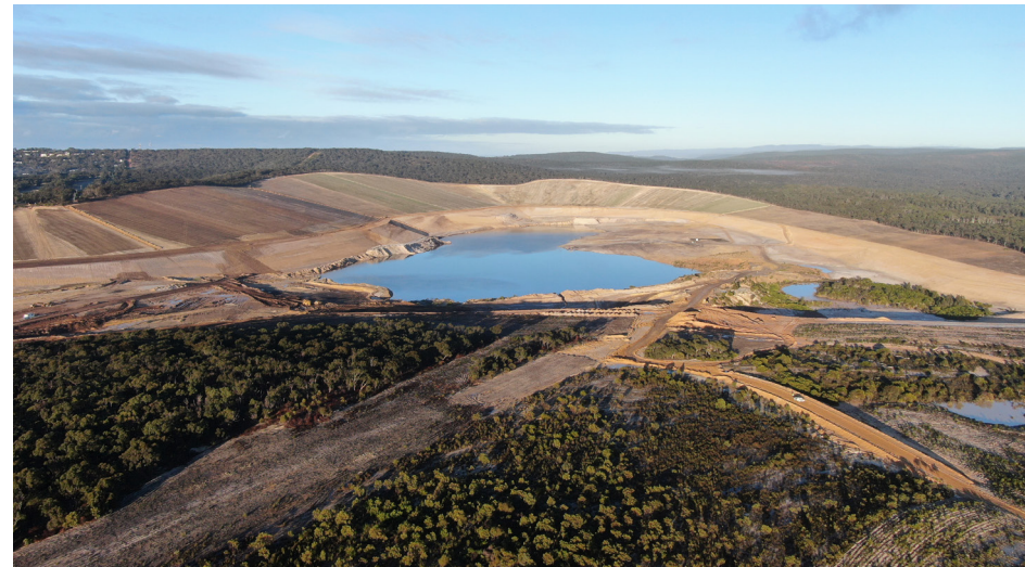
View towards the south-west corner of the mine showing the developing water body, the reprofiled south and west slopes and revegetation treatments. The grey strip in the foreground is the emerging vegetation on the former haul road.
